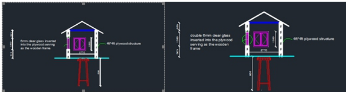
Figure 3.2: sketches of the field study for both the single glazed and the double glazed unit
