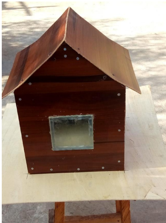
Plate II: Miniature model with double glazed unit. Plate III: kestrel weather meter mounted on a tripod stand.
